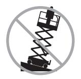
Do not raise the platform unless the machine is on a firm, level surface.
